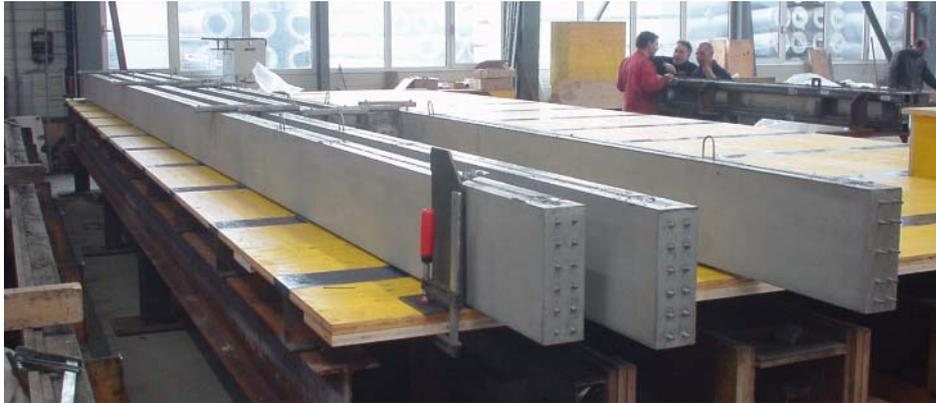
Fig. 4 11.1 m long (first two from the left) and 7.6 m long CFRP prestressed HPSCC facade beams
