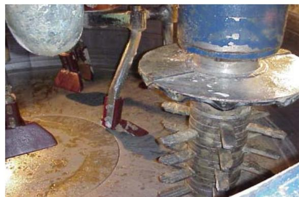
Figure 3: Wirbler and scraper installed
