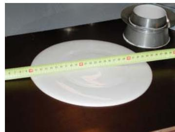
Figure 2c: The flow of the paste measured.
